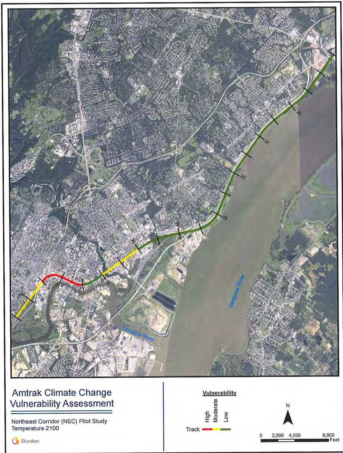
Figure 29. Linear Asset Vulnerability to Temperature 2100
