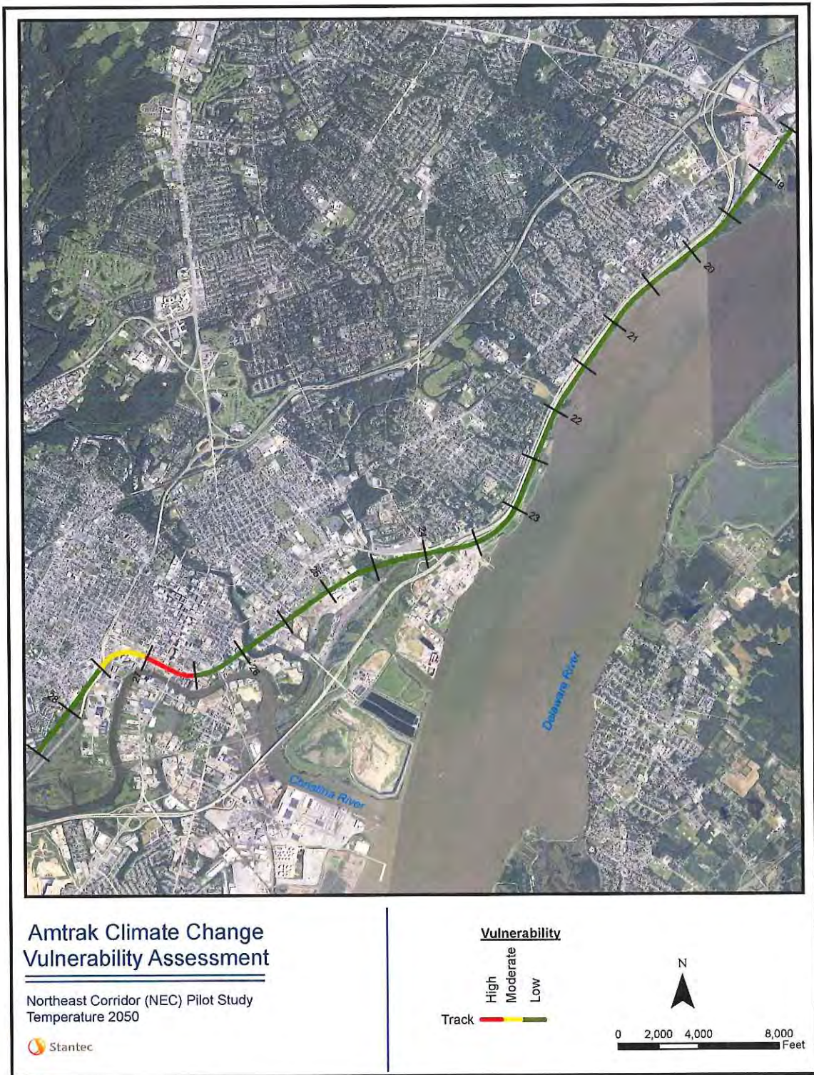
Figure 28. Linear Asset Vulnerability to Temperature 2050
