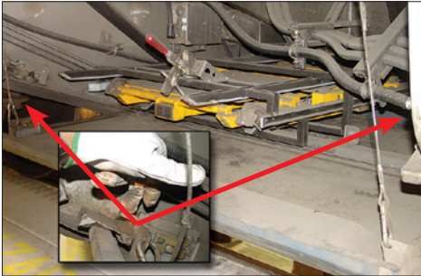
Figure 1-12 – Lower storage compartment latches and safety cables
