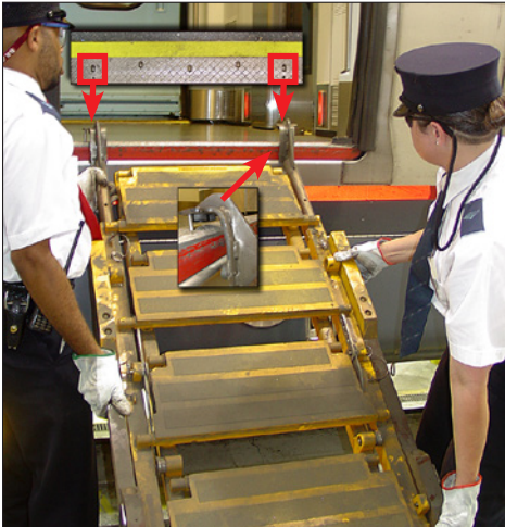
Figure 1-14 – Secure folding stairs to car body
