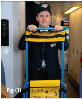
Fig (1) Grip both sides of extension handle, then pull up until it locks in place.
