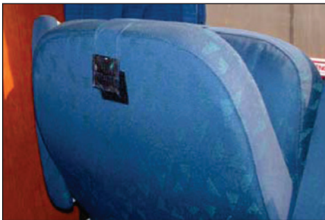
Figure 12-7 – Velcro Fabric Strap Securing Seat Cushion in Folded Position
